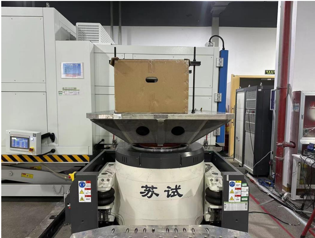
Fixed photos of Z-axis Random vibration (packaging) vibration
