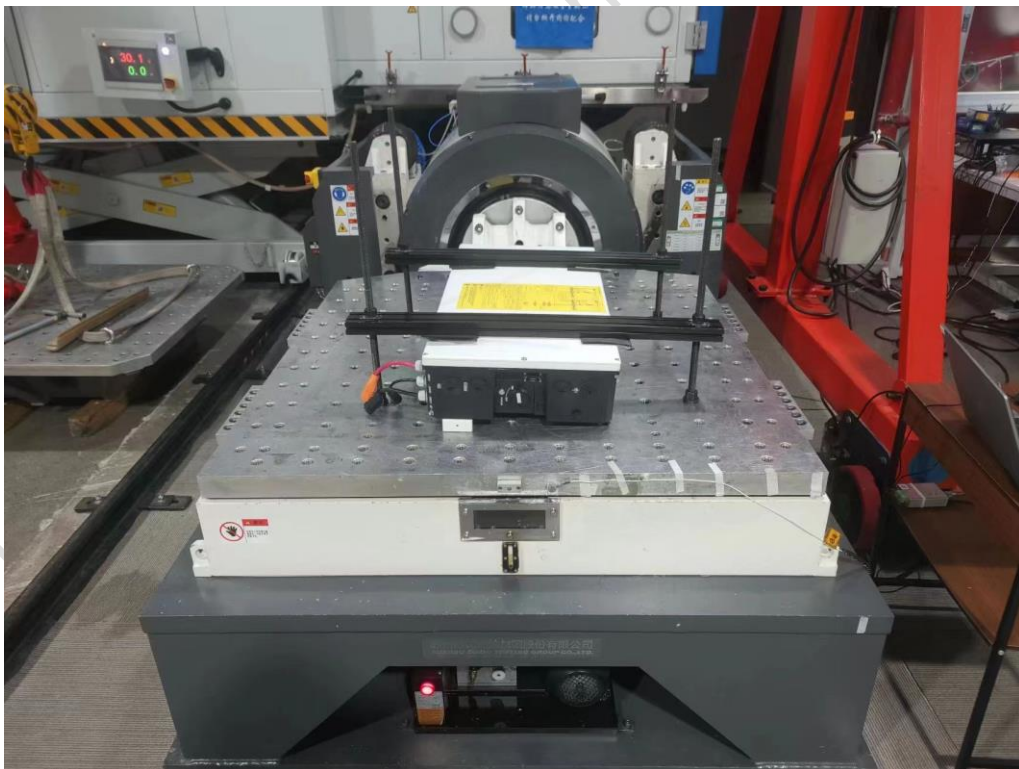
Fixed photos of Y-axis Sinusoidal vibration (bare machine) Random vibration (bare machine) vibration
